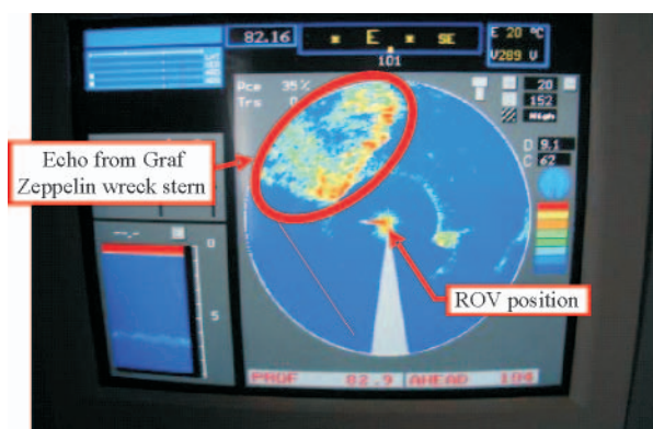
Fig. 3. ROV service desk in operation: sonar screen. Echo from the stern of the examined underwater object and vehicle position with respect to it are clearly visible (photo: S. Lipiński)
