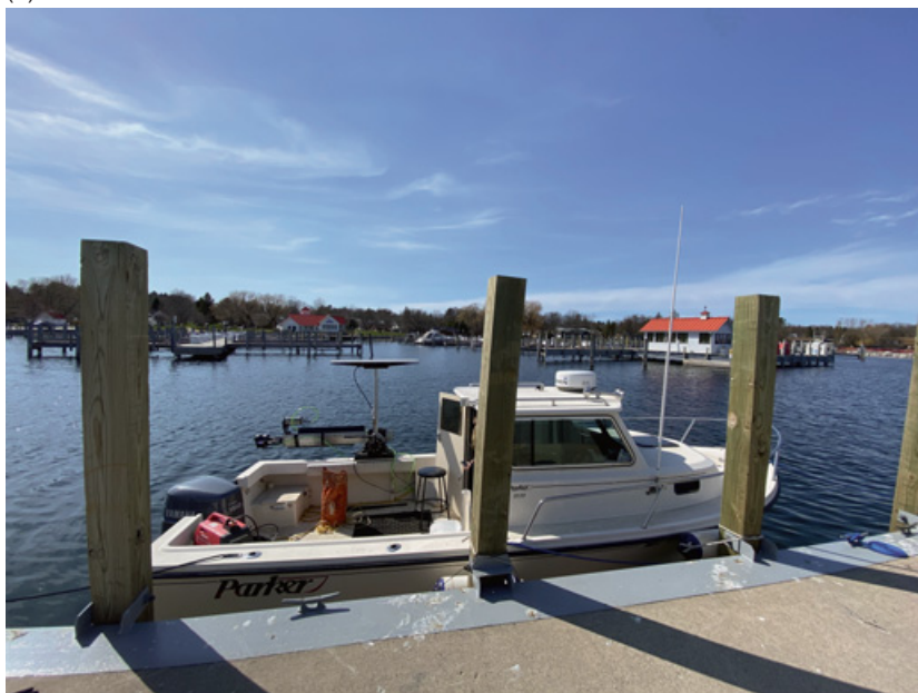
Figure 12 Multibeam SONAR installed on a 6.4 m Parker, Traverse Bay, Lake Michigan, Great Lakes, USA. (a) View of the M3 Multibeam SONAR Portable Hydrographic System, Kongsberg. This multibeam system is designed for shallow water applications not to exceed 50 m in depth. (b) Overview images of the SONAR and the vessel. Photographs by the author.
