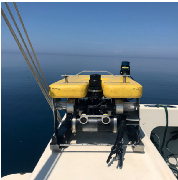
Figure 15 Outland 1000 remotely operated vehicle (ROV) Jake equipped for submerged site survey and mapping on the Alpena-Amberley Ridge, Lake Huron, Great Lakes, USA. Two red laser pointers installed on the front of the ROV provide scale. Photograph by the author.
