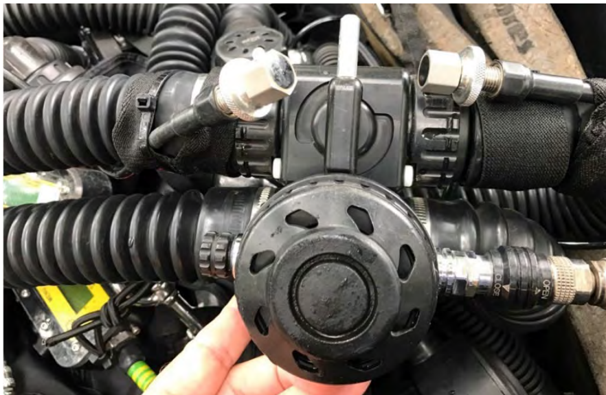
Figure 6. The dual BOV developed by Harris and colleagues for use in the Pearse Resurgence. The upper lever switches between loops and may be used to equalize them. The second control, not visible behind the OC second stage, allows bailout onto OC. This device makes the necessary task of switching between loops very simple, at the expense of a small decrease in redundancy. Photo courtesy Richard Harris.
