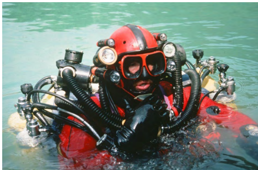
Figure 1. The RI 2000 rebreather used by Isler for his Doux de Coly exploration used two symmetrical backmounted semi-closed rebreathers with a third chestmounted unit. Photo courtesy Olivier Isler.
