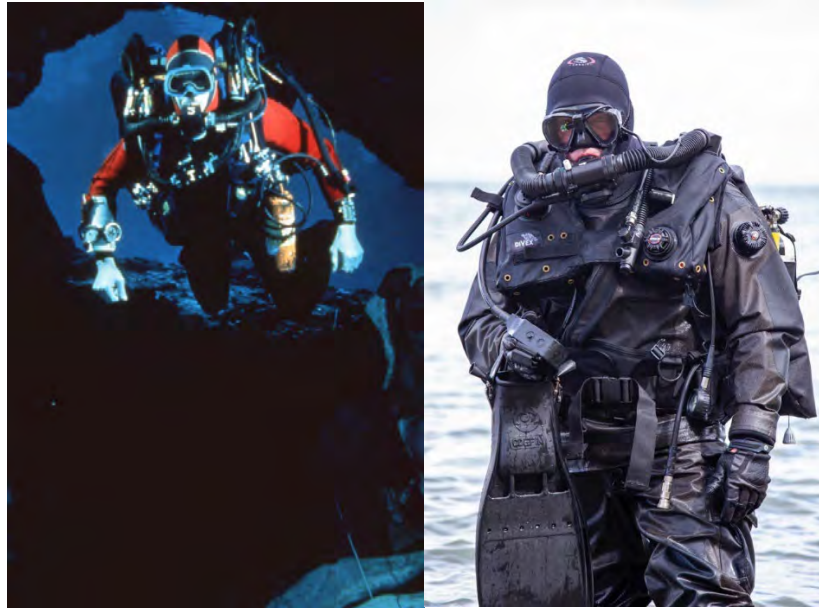
Figure 5. CCRs, the ultimate mixed gas platform. Photos courtesy USDCT and JFD Global ( https://www.jfdglobal.com/products/commercial-divers-equipment/rebreathers ).
