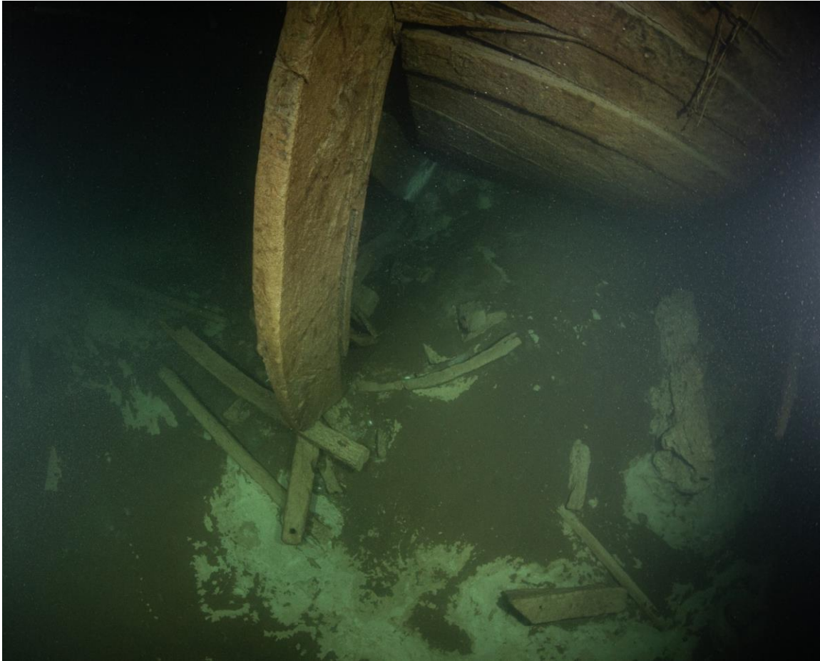
Figure 7. The stempost resting on debris from the wreck. Notice the cut-in in the lower part of the post for connecting two parts of the post (Jouni Polkko 2020).
