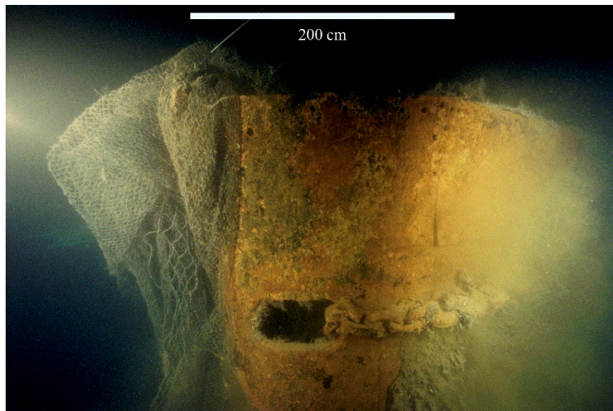
Figure 3. Trawler net damage on the AE2 submarine.
