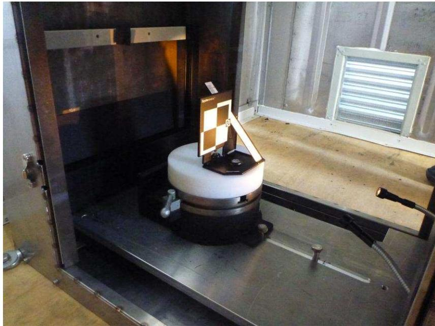
**Figure 12. Object placed on rotary stage. Photo by D. Creagh.**
