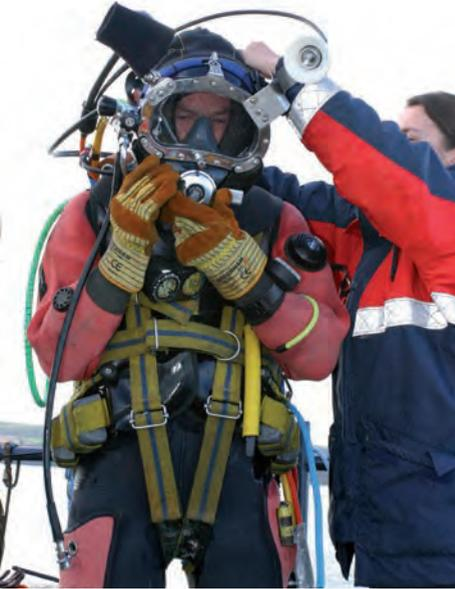
▲ © Wessex Archaeology. A diver putting on his equipment. Surface-supplied diver with the diving helmet and the umbilical device that supplies the diver with air; a communication line, video line to his/her camera, depth gauge, acoustic tracking and safety line.
