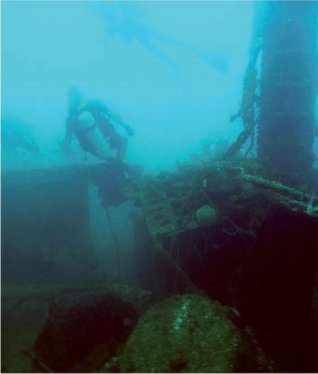
◀ B. Jeffery. A mooring block dropped onto the Kitsugawa Maru, causing considerable damage, Guam United States. While this poses a threat to the archaeological site, the navigational or environmental hazard of a wreck should be taken into account in its protection. In the illustrated case a site management plan should try to find a non disturbing solution for flagging the archaeological site to passing ships.
