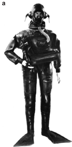
Fig. 31-10. (a) A diver wearing the pendulum closed-circuit oxygen rebreather used during World War II by Royal Navy X-craft divers. This rebreather was an adaptation of the Davis Submarine Escape Device (DSEA) manufactured in England by the Siebe-Gorman Diving Company. (b) Schematic diagram of a pendulum oxygen rebreather. The mouthpiece and hose, which connect the diver to the CO 2 scrubber, are a dead space in which carbon dioxide builds up during bidirectional ventilation. The diver exhales and inhales through a single hose connected to a CO 2 absorbent scrubber. The scrubber is built into a breathing bag (or counterlung) into which the diver exhales and from which he inhales. Fresh oxygen from the compressed gas supply below the breathing bag is added to compensate for metabolic consumption. The distal end of the scrubber is unused, while the proximal end adds to the dead space as absorbent is consumed. The rising concentration of carbon dioxide increases cerebral blood flow, thereby augmenting oxygen delivery to the brain and potentiating oxygen toxicity.
