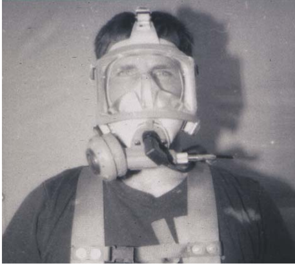
Fig. 31-8. The US Navy Mark 20 Mod 0 surface-supplied, open-circuit, lightweight system with full facemask is limited to a depth of 60 fsw for applications such as diving in mud tanks and enclosed spaces. Reprinted from US Department of the Navy. US Navy Diving Manual . SS521-Ag-PRO-010. Washington, DC: Naval Sea Systems Command. Rev 4 (20 Jan 1999); Change A (1 Mar 2001): p6-55. NAVSEA 0994-LP-100-3199.
