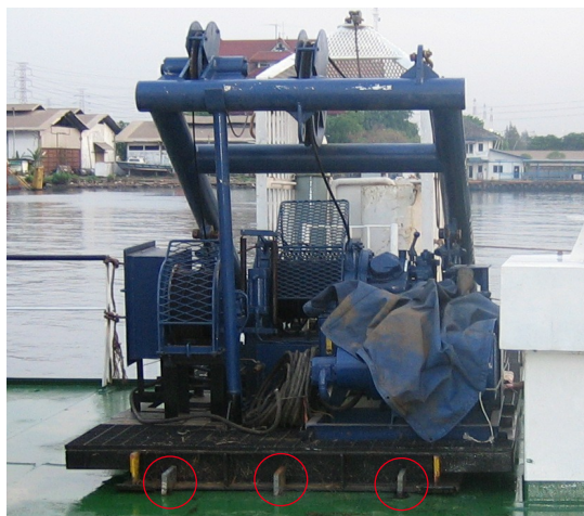
Wedges welded to the deck, but not the chassis
