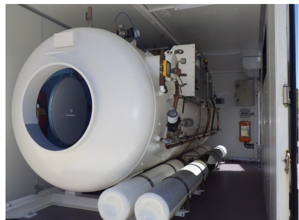
Surface-supplied diving chamber in an isolated container
