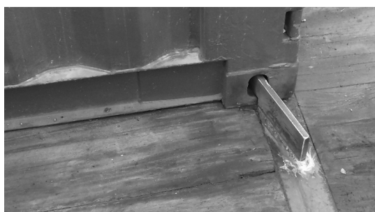
Welded wedge securing an ISO fitting
