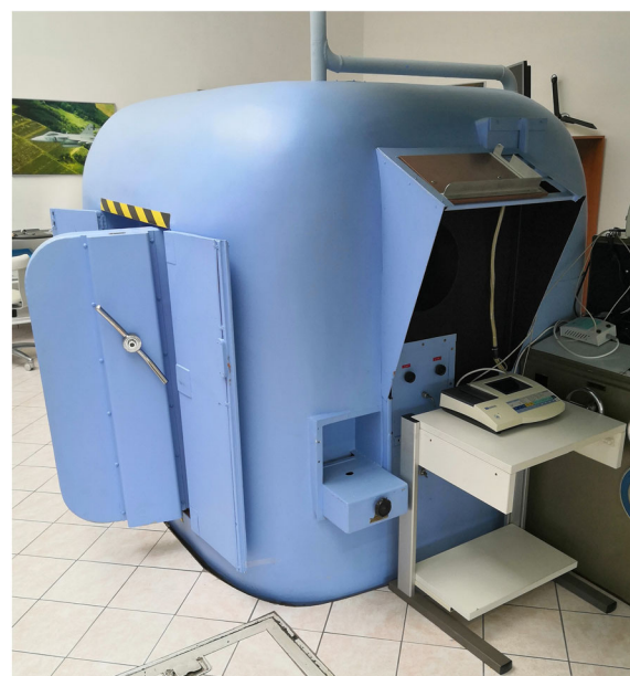
The hypobaric chamber for practicing explosive decompression.
