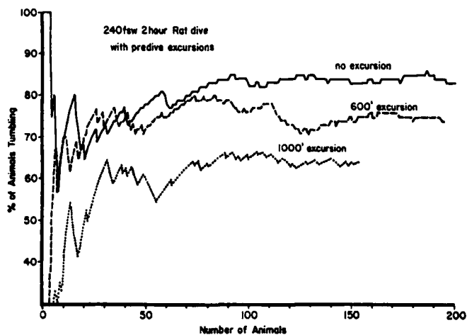
Fig. 7. Results of tests of Fig. 6; bends incidence (% of animals tumbling) is illustrated as a function of number of animals exposed.
