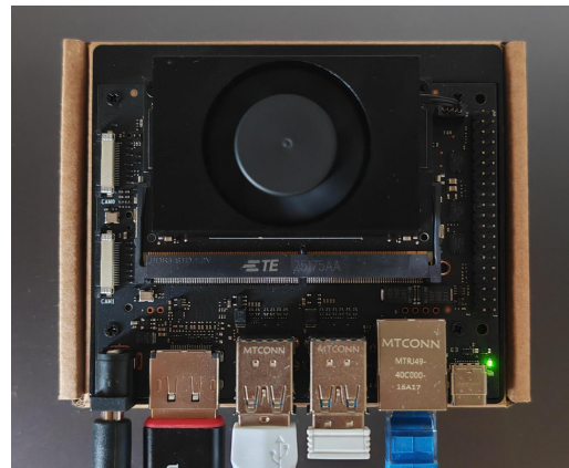
Figure 13. Embedded hardware platform used for deployment-oriented inference evaluation on NVIDIA Jetson Orin Nano.
