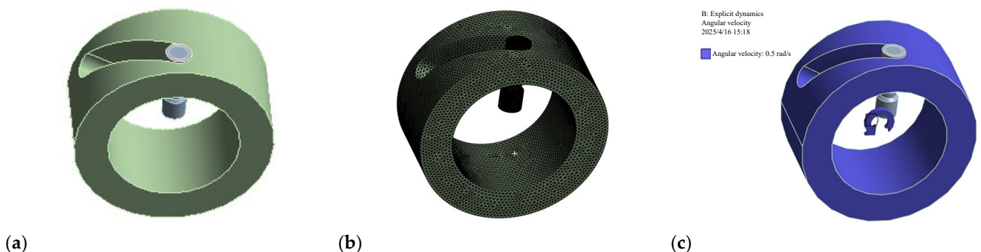
Figure 18. Finite element model for shear pin strength analysis. (a) Simplified model. (b) Results of finite element meshing for impact simulations. (c) Simulation boundary conditions under impact conditions.
