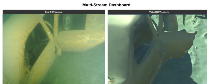
Figure 13. Real-time synchronization between the physical BlueROV2 camera feed and the digital twin's virtual perspective.
