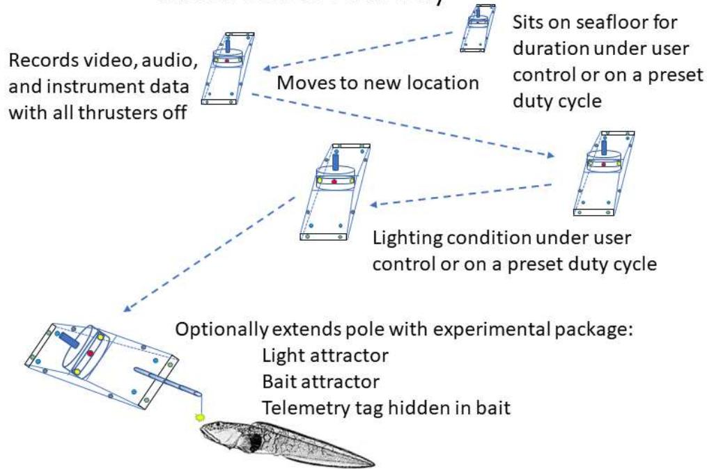
Figure 2. Typical operational scenario for a stealth ROV/AUV.
