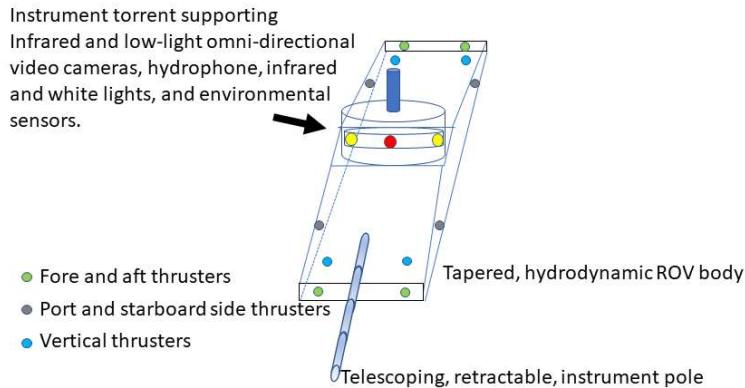
Figure 1. Concept of a stealth ROV.
