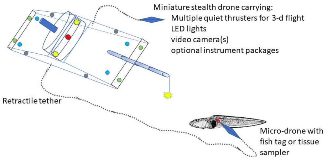
Figure 3. Stealth Mothership ROV with satellite micro-drones.
