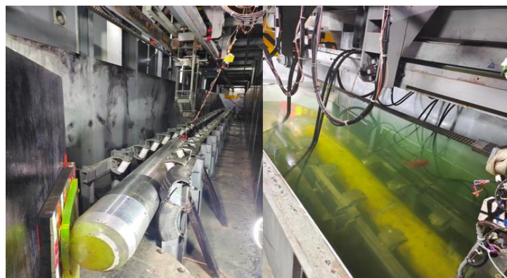
Figure 1. Physical model of UUV shell and test device
