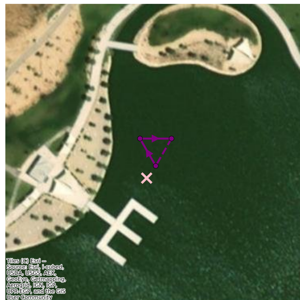
Figure 8. Example planned search polygon used in the acoustic localization experiments. The polygon vertices denote predefined listening locations visited sequentially by the PIRATE platform (solid arrows indicate traversal order). The dashed edge illustrates the closing segment of the polygon. The pink cross marks the ground-truth position of the acoustic tag, which was unknown to the system during mission execution.
