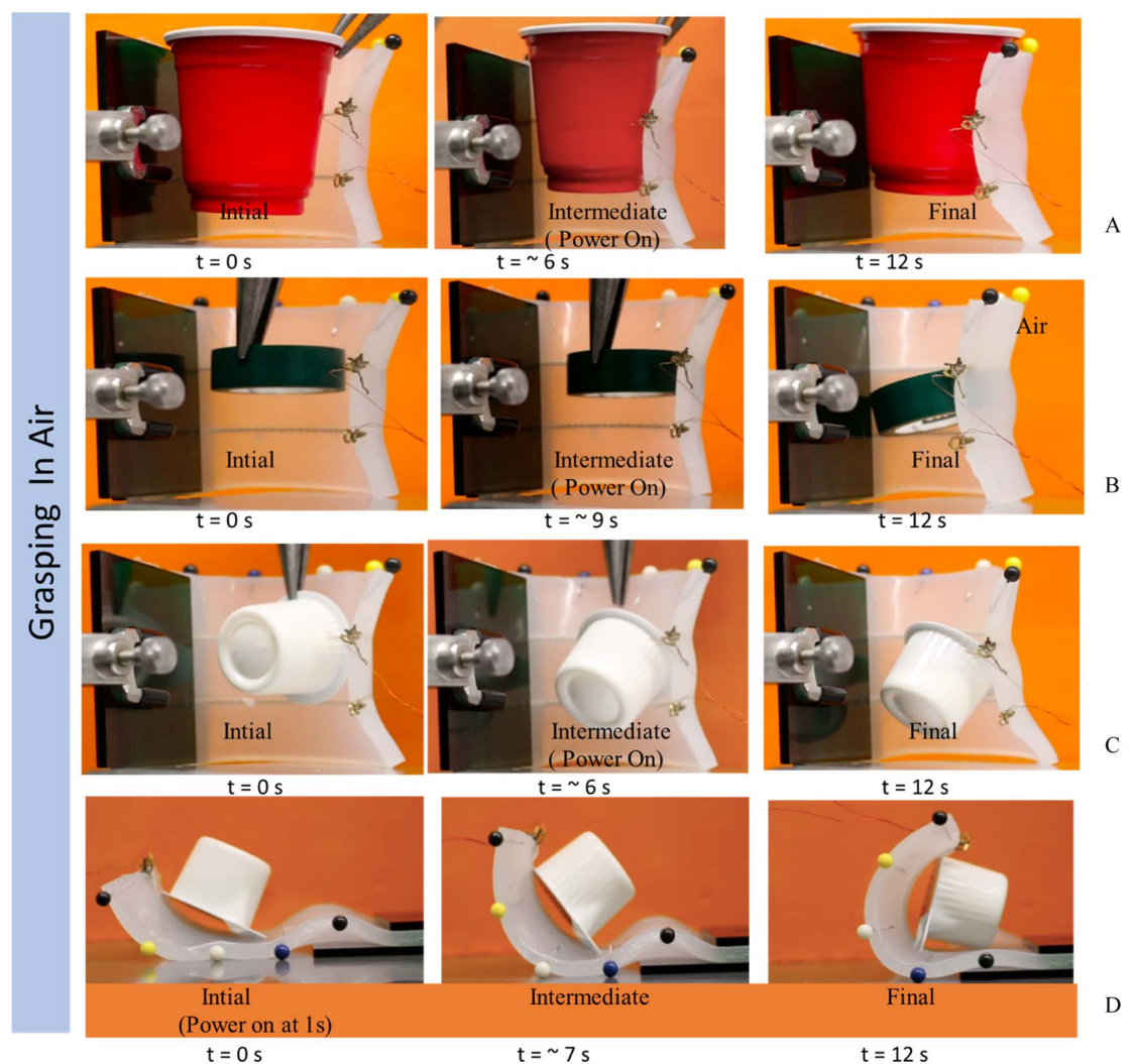
Figure 11. Vertical grasping of objects in air ((A) to (C), the top three rows), gravity is vertically downward and horizontal grasping of objects by keeping objects on the top of the skin with a single limb is shown at the bottom row (D). The intermediate steps shown in the second column for each row indicate the power on state (actuating the muscles) and the time variation is because we didn't focus on the powering time (on time), rather the holding of the object is the main goal of the experiment.
