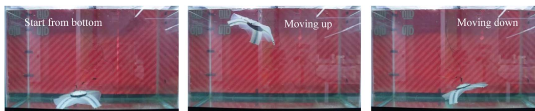
Figure 9. The above shown images display the swimming vertically up and down of the Quadralimb Bot 4.0 for 200 cycles.
