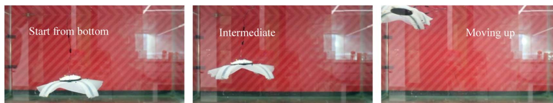
Figure 7. The above shown images display the swimming performance of the quadralimb Bot 3.0 for 100 cycles.
