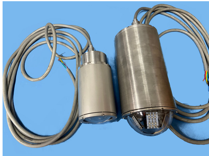
FIGURE 9 Prototype: receiver on the left and transmitter on the right.
