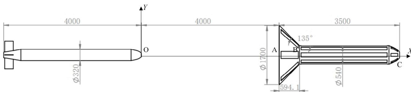
Figure 1. AUV underwater docking numerical model.
