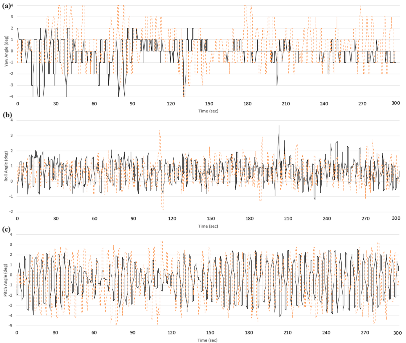
Fig. 17. Sensor values to assess vehicle stability before and after the integration of the manipulator: (a) Yaw, (b) Roll, (c) Pitch.
