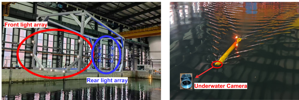
Figure 14. The docking station with dual-layer light array and TS-MINI AUV of SIA.
