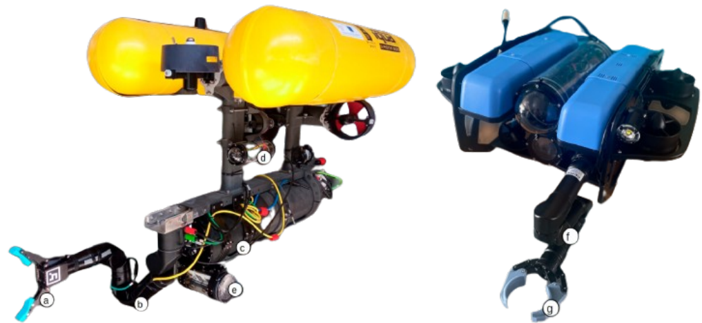
Figure 5. On the left the G500 I-AUV. (a) Two-fingered end-effector with camera, (b) Reach Bravo 7 manipulator, (c) Payload enclosure, (d) Low-Light HD USB camera enclosure, (e) Jetson Orin and stereo camera enclosure. On the right, the BlueROV I-AUV. (f) Reach Alpha 5 manipulator, (g) Custom end-effector for pipe grasping.
