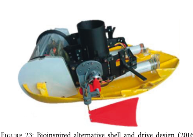
FIGURE 23: Bioinspired alternative shell and drive design (2016) [29].
