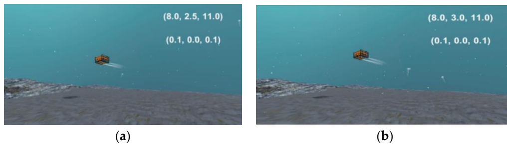
Figure 19. Multi-group depth target test effect. (a) Test effect with target depth of 2.5 m. (b) Test effect with target depth of 3.0 m.
