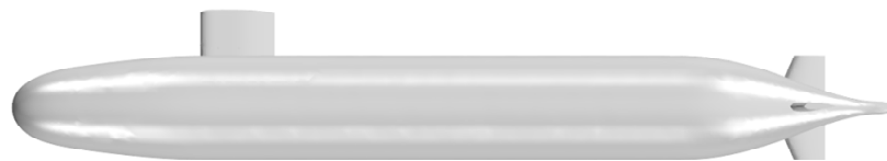
Figure 5. Full-body SUBOFF geometric model.
