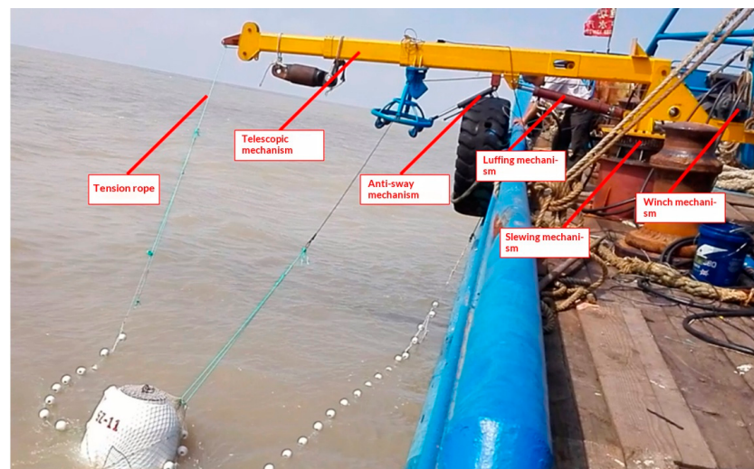
Figure 1. Harsh sea state marine cranes.
