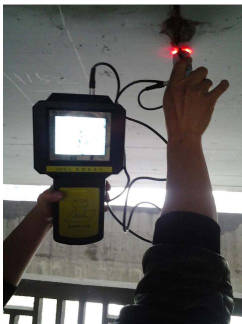
Fig 15. Crack width detection.
