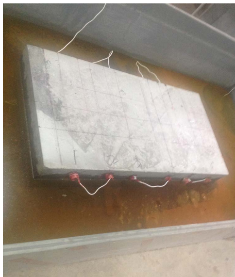
Fig 11. Reinforced concrete slab energized corrosion test.
