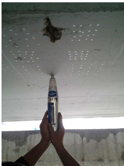
Fig 16. Concrete strength test.
