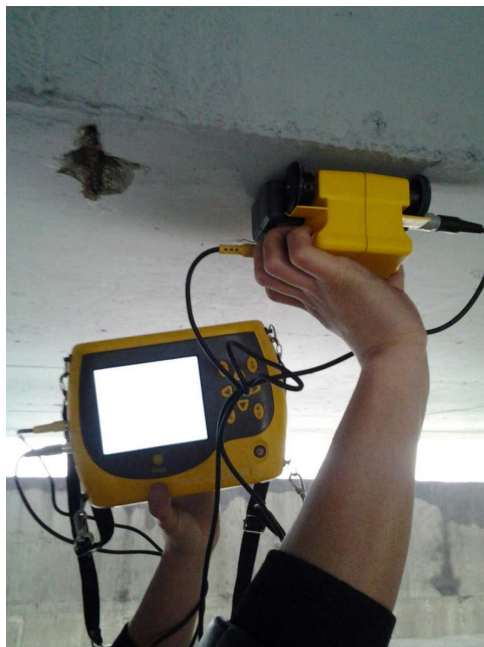
Fig 17. Testing of concrete protective layer.
