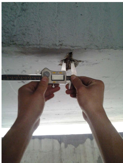
Fig 18. Diameter test of corroded steel bars.
