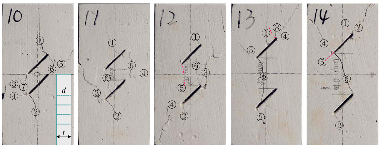
(c) Surface crack features of specimens 10# ~ 14#, d/t = 1
