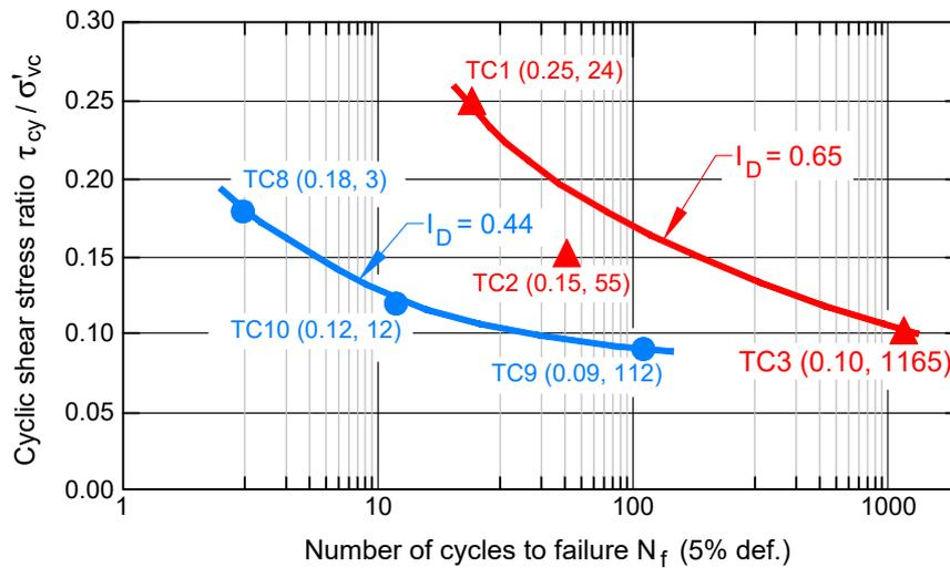
Figure 6.18 : Curves of cyclic shear strength of the N34 Fontainebleau sand for two density indices, with  $N_f$  = number of cycles leading to liquefaction, defined for 5% of axial strain of the sample (from SOLCYP, 2017)
