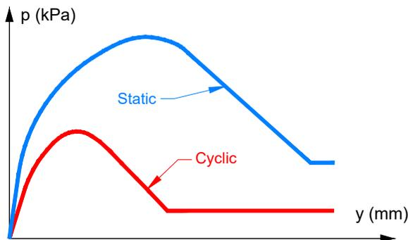
Figure 9.13: Static p-y curves (overconsolidated stiff clays)
