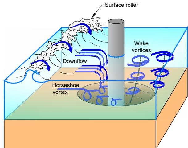
Figure 11.6 : Mechanisms causing scour around a monopile
