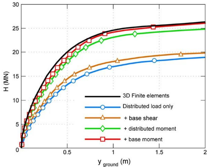
Figure 8.5: Impact of the 4 elements of the ground response on the lateral load curve  $H$  in function of the lateral displacement  $y$  of a very short monopile (penetration length = 2 diameters) in a sand (from Byrne et al., 2015)
