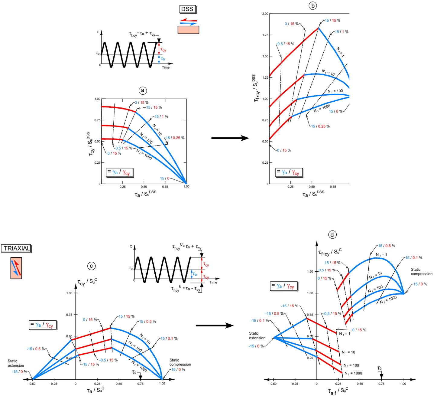
Figure 10.5: Examples of representation of the degradation of shear strength for the whole spectrum of cyclic loading and for different number of cycles, under DSS (a and b) and Triaxial (c and d) loadings, (from Andersen et al., 2013)
