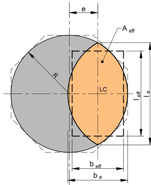
Figure 10.2: Effective cross-sectional area of a circular foundation
