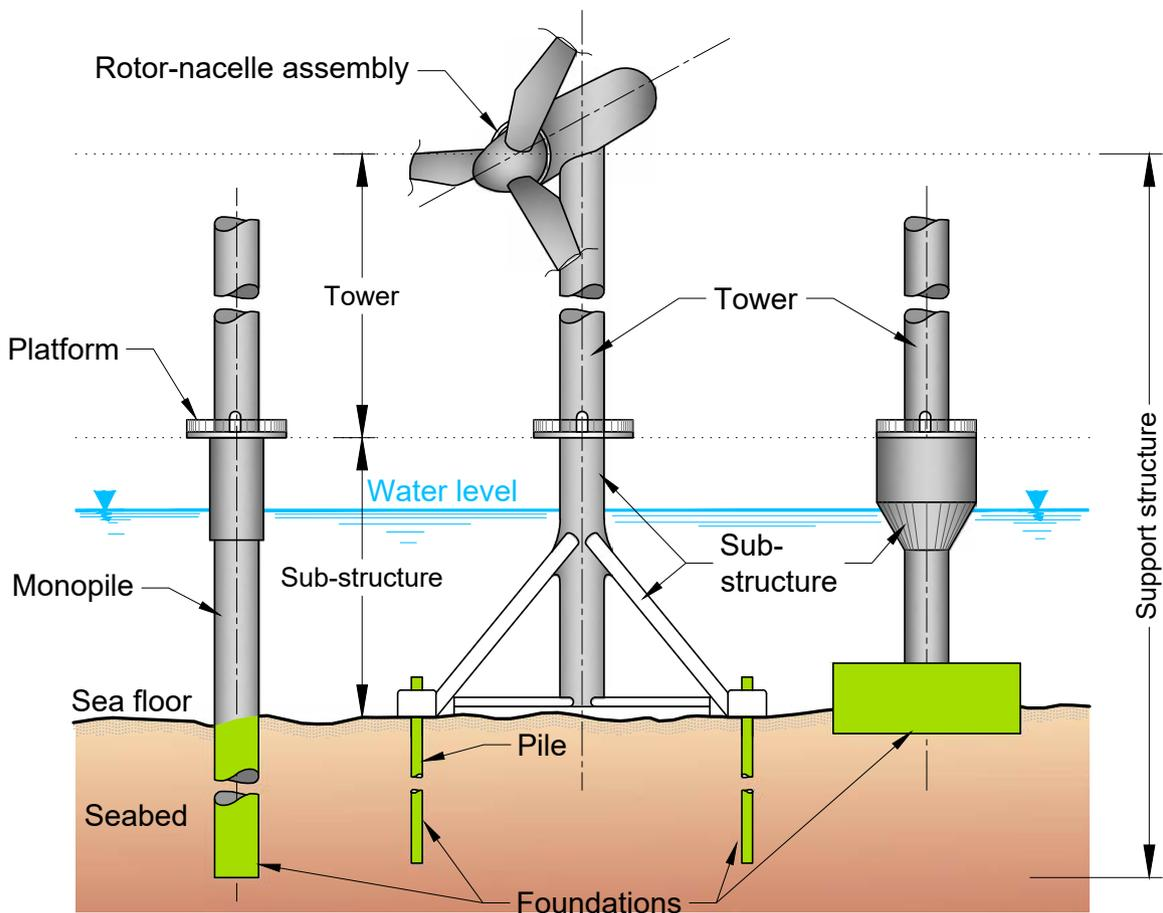
Figure 1.1 : Components of an offshore wind turbine
