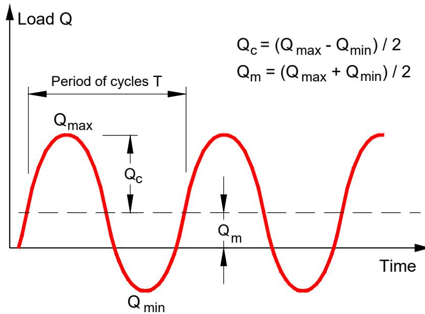
Figure 4.1 : Definitions for a regular cyclic loading
