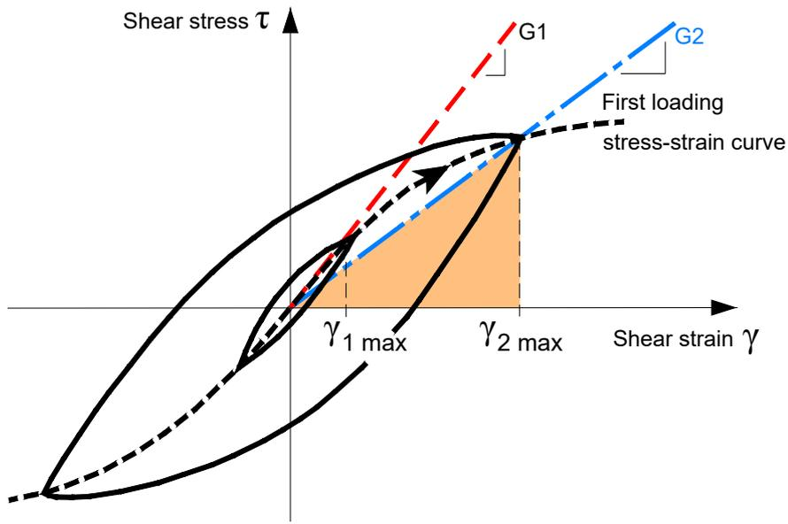
Figure 6.2 : Centred cyclic loading – Direct simple shear test
