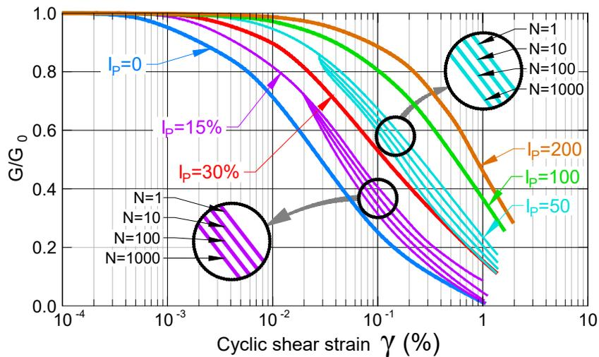
Figure 6.20 : Variation of the normalized shear modulus  $G/G_0$  in function of the level of cyclic strain  $\gamma_{cy}$  for a normally consolidated soil (with a consolidation stress below 150kPa) showing the effect of the plasticity  $I_p$  and of the number of cycles  $N$  (from Vucetic et Dobry, 1991)
