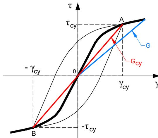
Figure 6.10 : Definition of the shear moduli
