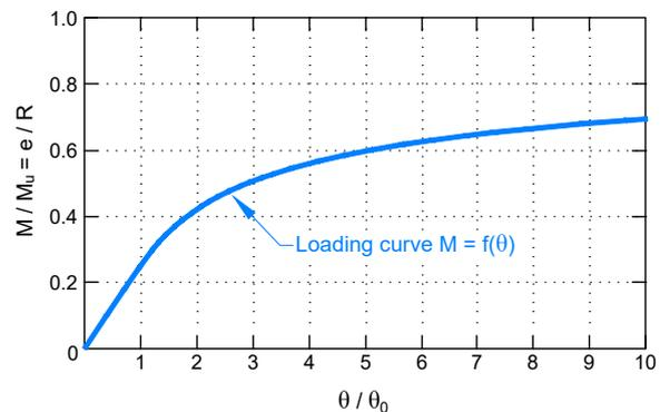
Figure 10.7: Normalised moment-rotation curve – Circular foundation
