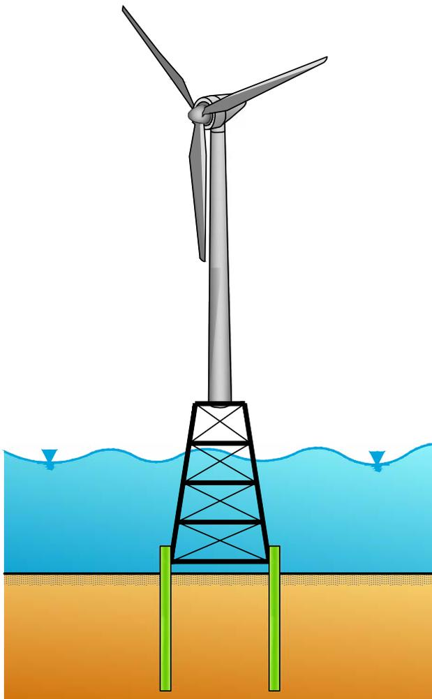
Figure 9.1: Jacket support of a wind turbine – Principle
