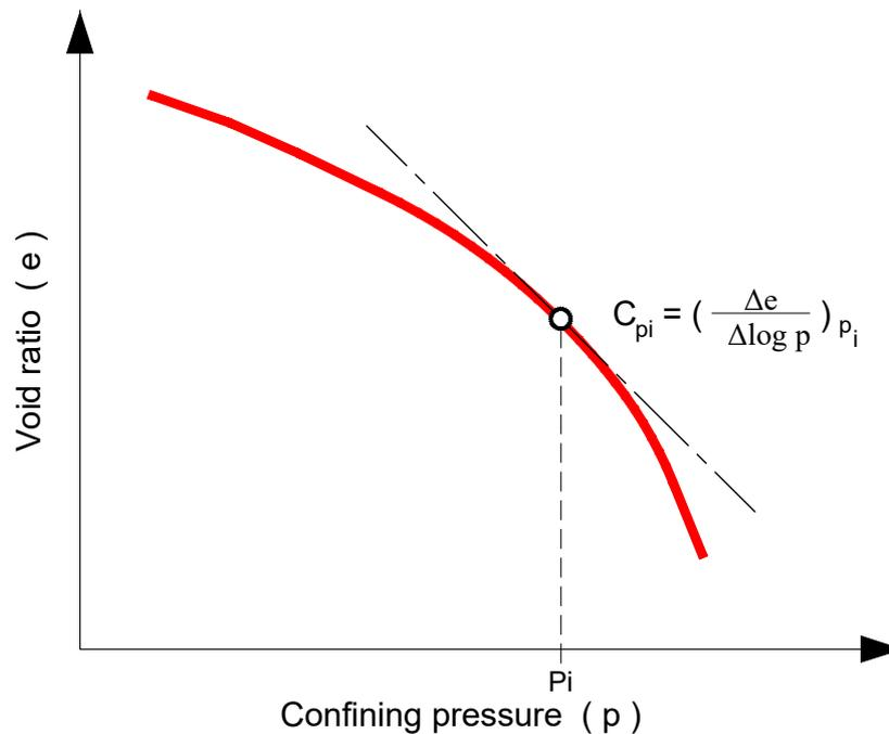
Figure 9.6: Definition of the tangential compressibility index
