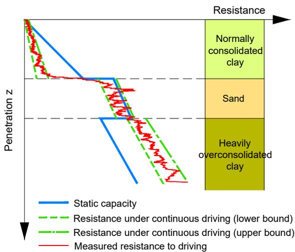
Figure 9.29: Components of the SRD during continuous driving
