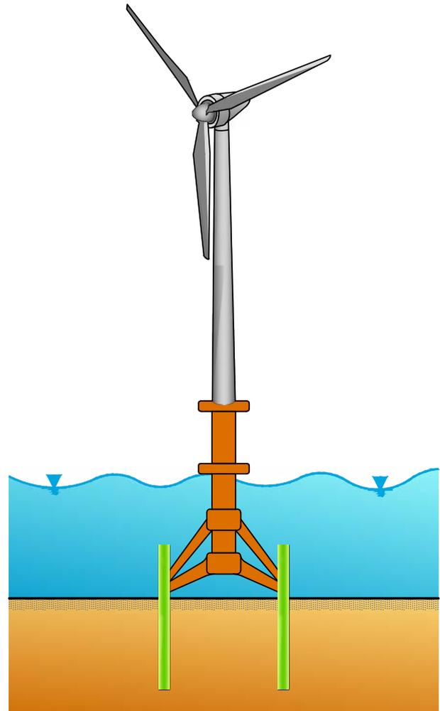
Figure 9.2: Wind turbine support of the tripod type
