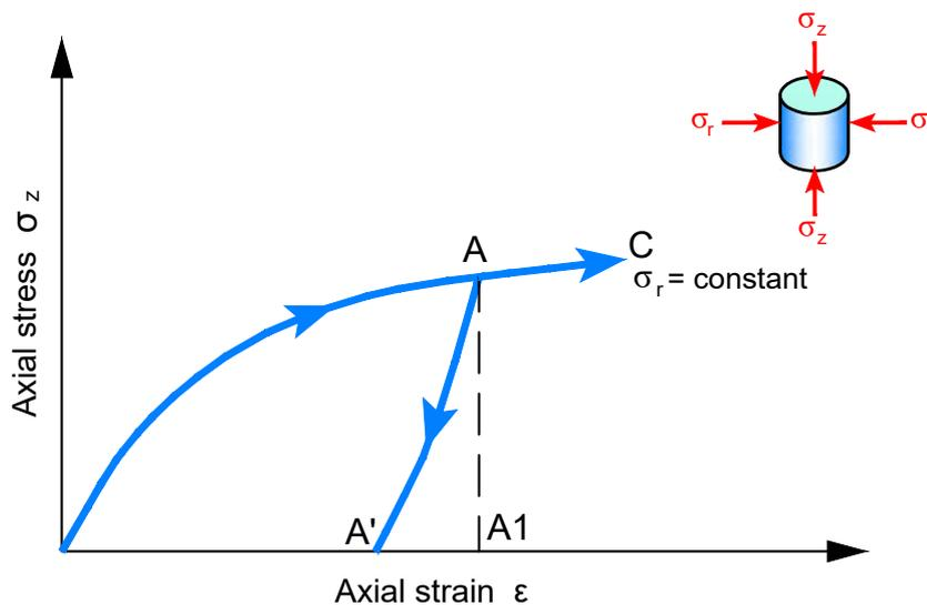
Figure 6.1 : Stress-strain curves under a quasi-static monotonous loading
