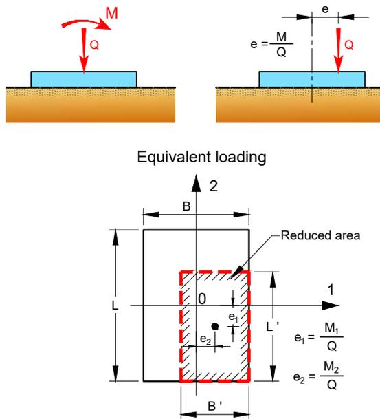
Figure 10.1: Effective cross-sectional area of a rectangular foundation
