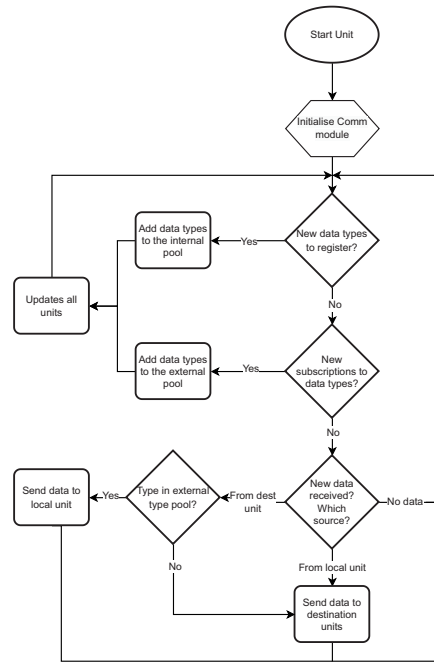
Fig. 1. Flow chart of the communication module.
