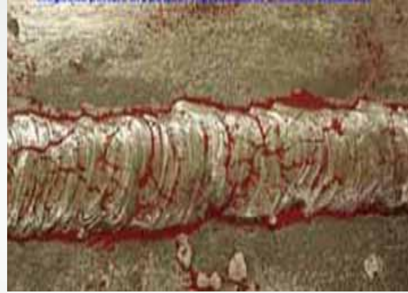
Indication of cracks in a weldment
