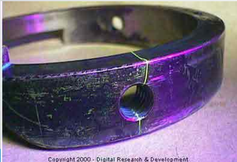
Magnetic particle wet fluorescent indication of a cracks at a fastener hole
