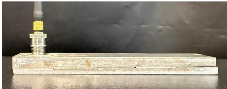
Figure 3. Experimental setup for corrosion monitoring benchmark.
