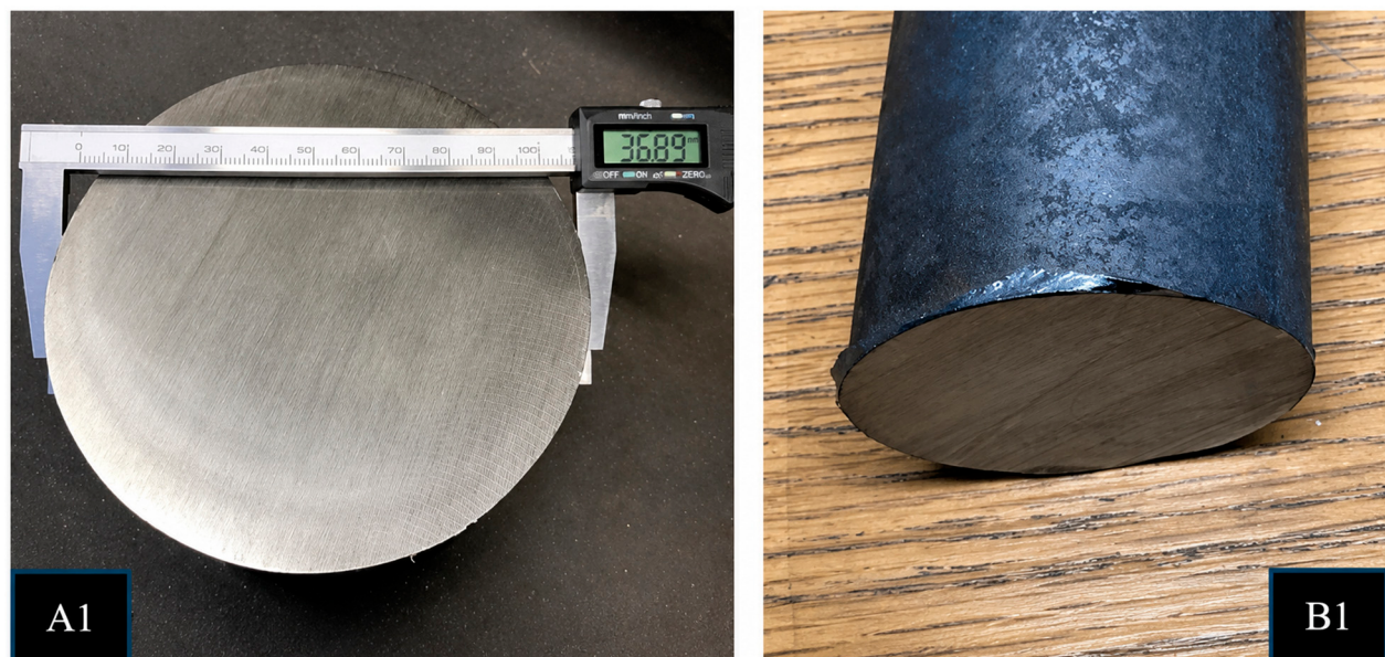
Figure 1. Digitally measured bulk material diameters prior to machining and specimen extraction: A1—AISI 316 ( D = 369 mm) and B1—AISI 304L ( D = 50 mm). The figure documents the original section size and sampling provenance, ensuring dimensional traceability between bulk material, destructive testing specimens, and subsequent non-destructive evaluation.
