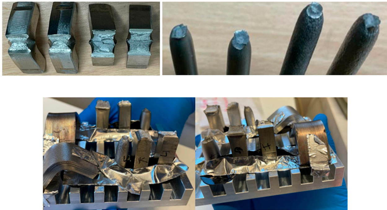
Figure 2. (Top) Cross sections of fractured Charpy V-notch specimens (A1, A2, B1, B2) and fractured tensile specimens (B2, B1, A2, A1). (Bottom) Representative broken specimens positioned for SEM loading. The figure establishes specimen-level traceability between mechanical testing and fractographic analysis within the integrated DT+NDT workflow.
