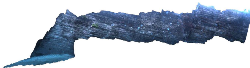
Fig. 15. A 3D map generated from 350 stereo based point clouds from a Bumblebee camera on a Sparus vehicle of the University of Girona. The consistently dense stereo data in all stereo computations indicates high rectification accuracy.
