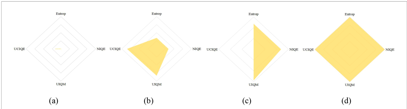
FIGURE 10 Normalized quantitative assessment of each version using the Entropy, NIQE, UIQM, and UCIQE metrics. (a) Raw underwater image (b) w/o RB (c) w/o Ab (d) UIVE.
