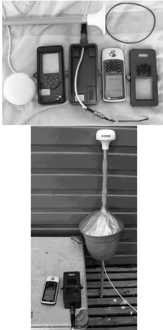
Figure 10.1. Complete underwater GPS system.
