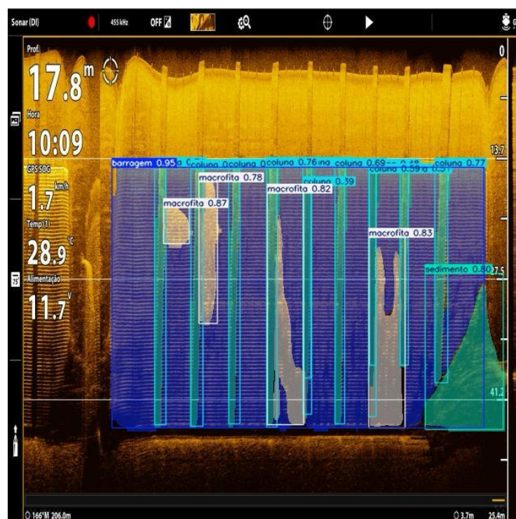
Figure 3. Post-processed sonar imagery of a hydropower trash rack.
