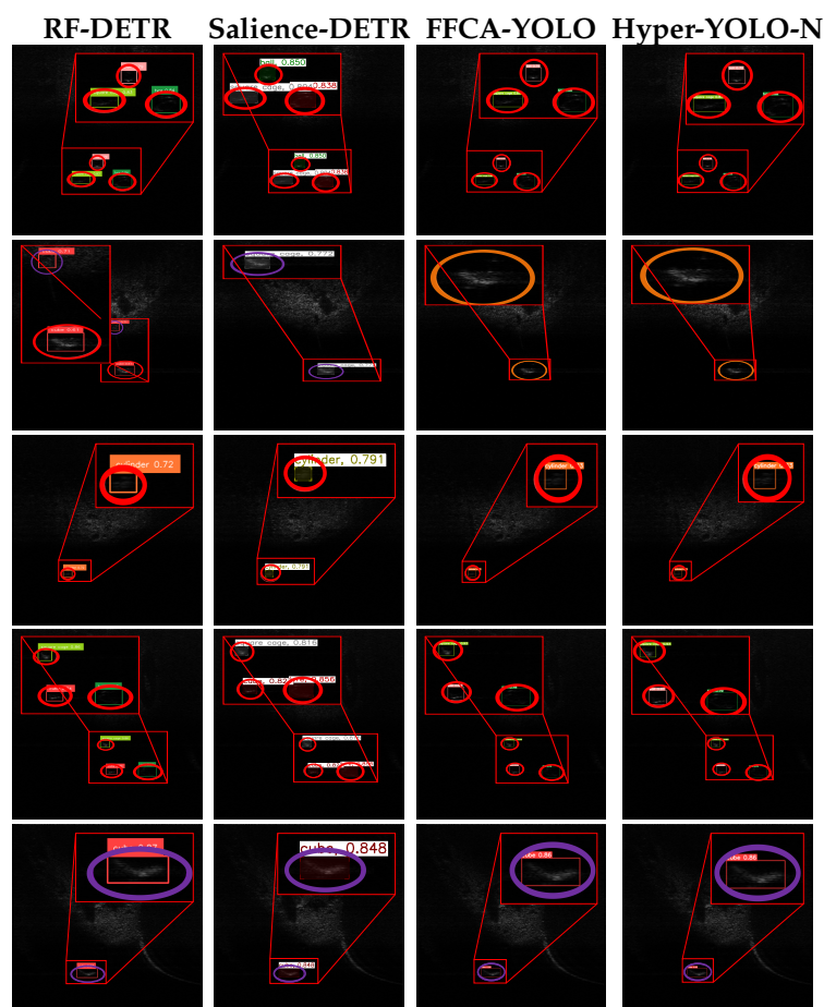
Figure 9. Qualitative detection results obtained by representative SOTA methods on the UATD-Test-1 dataset. Red, orange, and purple circles denote true positives, missed detections, and false alarms, respectively.
