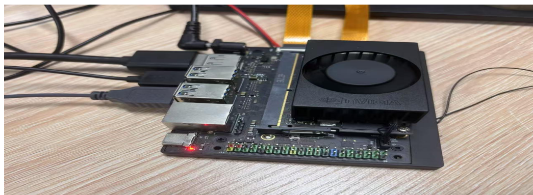
Figure 10. Embedded runtime validation setup of the proposed method on the NVIDIA Jetson Orin NX platform.
