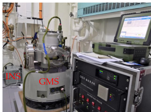
Figure 7. Shipborne gravity-assisted navigation system.
