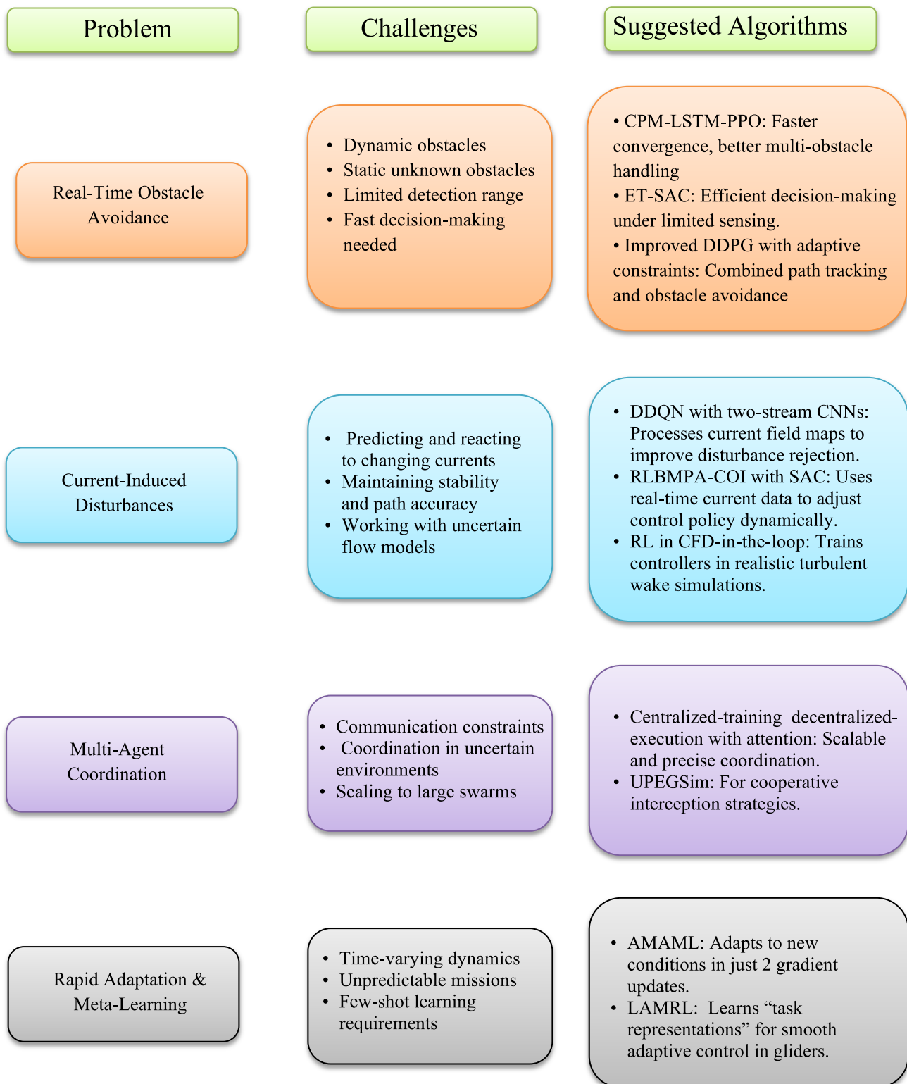
Fig. 4 Presents the problems, which faced the reinforcement learning and suggested algorithms to solve it
