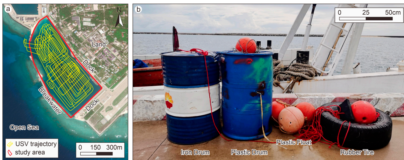
Figure 4. Harbor location and simulated seabed objects. (a) Satellite remote sensing image of the island harbor, showing the Harbor layout with infrastructural features. The survey trajectory of the USV is indicated by the yellow line; (b) Deployed simulated objects, from left to right: iron drum, plastic drum, and rubber tire.
