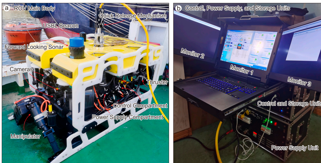
Figure 3. Main Components of the “Dolphin II-A” ROV. (a) ROV submersible unit. (b) Deck control console.
