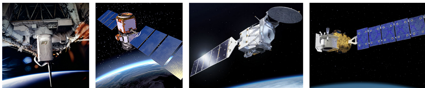
Figure 5. The selected deployment platforms carrying LiDAR instruments, from the left: LITE instrument on top of the Space Shuttle Discovery, CALIPSO satellite carrying a CALIOP instrument, EarthCARE carrying ALTID and ICESat-2 with ATLAS instrument [112–115].
