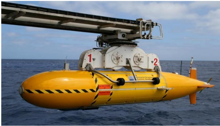
Fig 3: A typical AUV ready to be deployed
