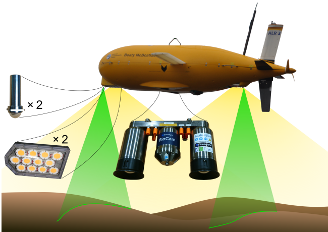
FIGURE 6. BioCam setup on ALR. The main housing containing the the cameras and electronics is mounted centrally. Sheet lasers and LED strobes are mounted one each at front and the back of the vehicle.
