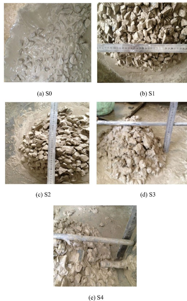
Figure 4. Cohesiveness and water retention of artificial reefs with different material ratios [51].
