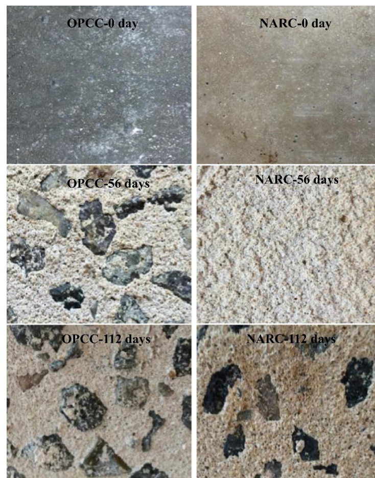
Figure 7. Surface images of NARC and OPCC attacked by biological sulfuric acid [58].
