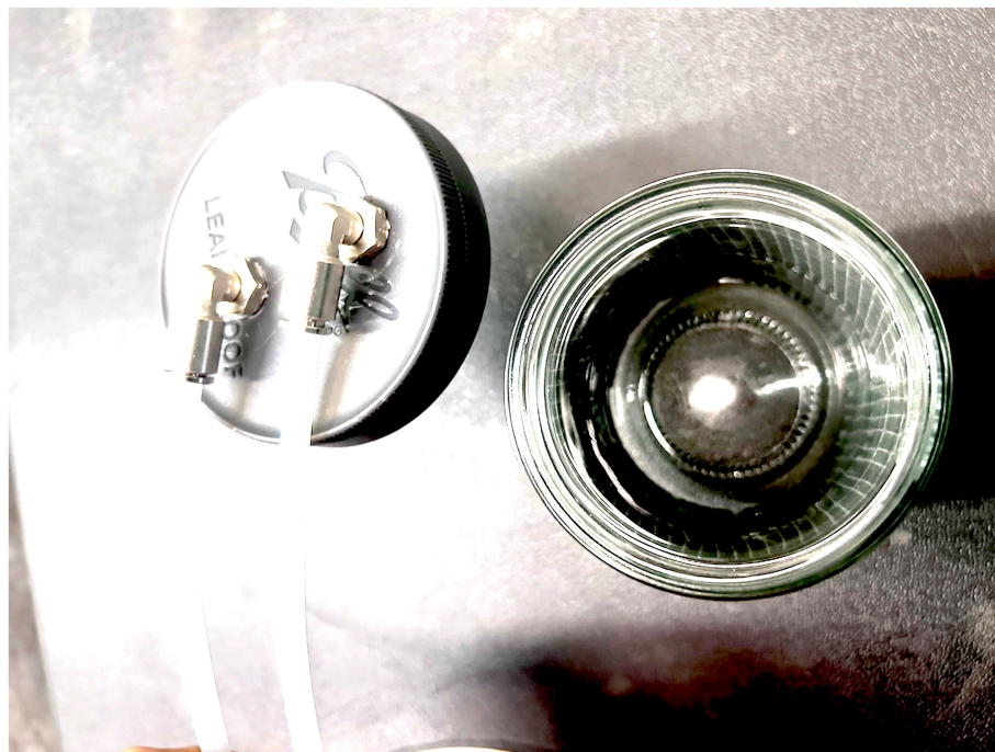
FIGURE 4 Part #5 Glass Mason jar, which holds the target sample.
