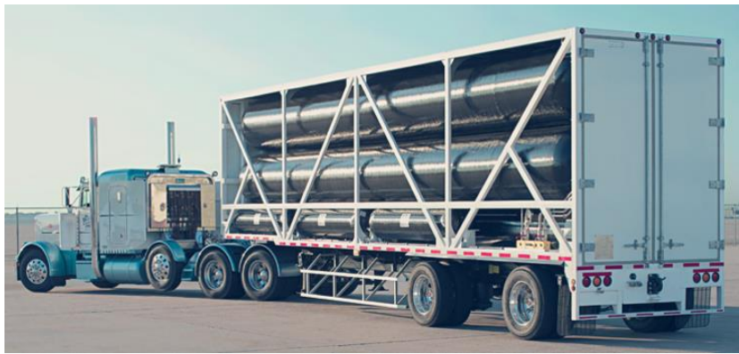
Figure 2. MEGC containing tubes linked to each other
