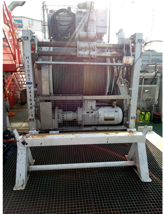
Winch of the WR 200 ROV installed on the rear of the horizontal chassis. Note the steel wire wrap of the umbilical.
