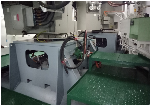
Upper parts of the tunnel thrusters of UDS Lichtenstein
