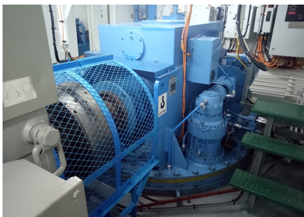
Topside parts of Azipull: Starboard side.
