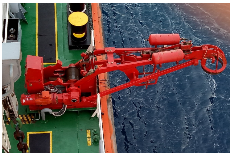
Taut wire deployed (at work)
