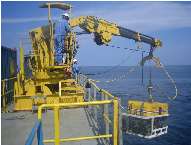
Crane starting to lower a ROV to the water (it is a old model). Note that the umbilical is not used to lift the machine.
